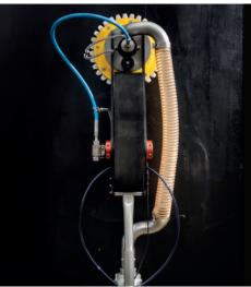
Compact magnetic cleaning and paint-stripping solution designed for closed operations. The VertiDrive M2 is a solution for fast and efficient removal of coating, rust and all sorts of contamination vertically, horizontally or overhead. The machine adheres to the surface with permanent magnets, absorbing all energy from the water pressure, up to 2500bar/ 36.000 psi.
